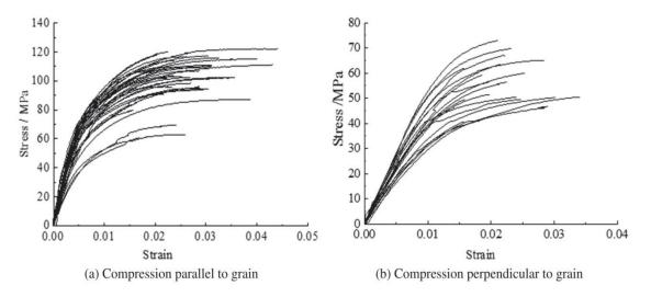
Figure 8: Stress and strain curves for compression specimen [75]
