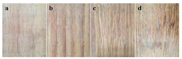
Figure 6: The surface of bamboo scrimber with different textures (a wood grain; b strip-shaped; c mountainshaped; d pattern of vortexes) [7]
