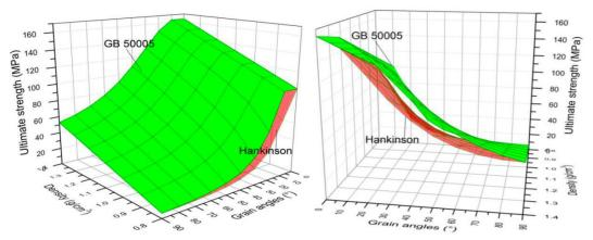
Figure 10:2D models of ultimate strength for various grain angles and different densities Figure [85]
