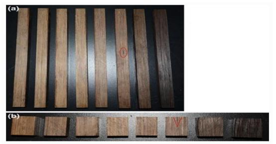
**Figure 12**:Discoloration of the control and heat-treated bamboo scrimber samples. From left to right are the control samples and samples exposed to 50, 80, 110, 140, 170, 200, and 230 °C for 2 h. a Bending sample. b Compression samples [60].
