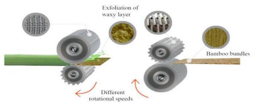
Figure 5:Schematic diagram of the novel fluffer machine developed by the Chinese Academy of Forestry [7]
