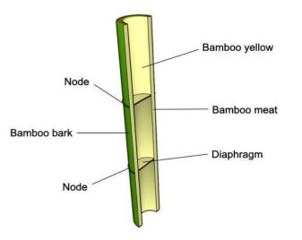
Figure 1: Basic geometric features of a bamboo culm
