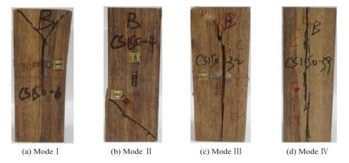
Figure 9: Typical failure modes for axial compression specimens[75]
