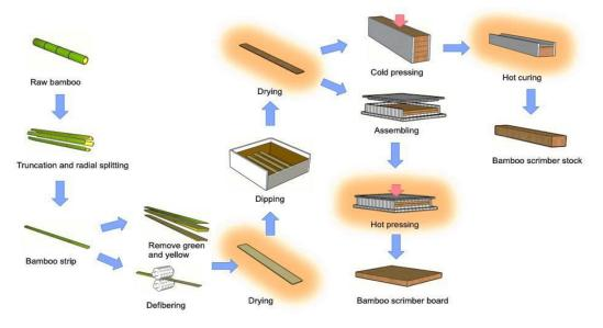
Figure 4: Process flow diagram of bamboo scrimber
