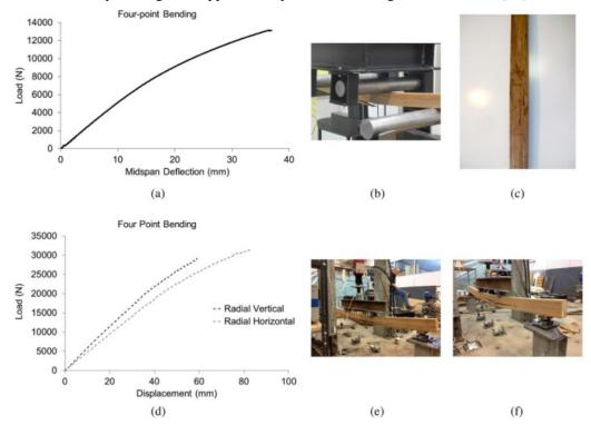
Figure 11:Four-point bending (a) results and (b) specimen failure for bamboo scrimber. Laminated bamboo (c) results and specimen failures for (d) radial horizontal and (e) radial vertical orientations [76]
